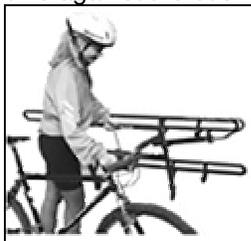
4. Lift your bike onto the bike rack, fitting wheels into labeled wheelslots. Each wheel slot is clearly labeled for the front wheel. (NOTE: The rack operates properly even if a bicycle is loaded in the wrong direction.) The purpose of the directional placement is to make the bike nearest the bus easier to unload.
